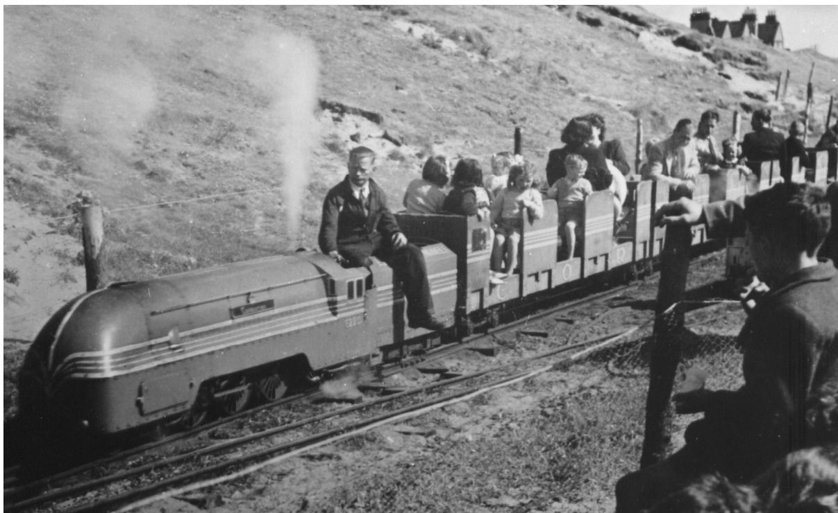
This view of "Coronation" hauling a well-loaded train at Prestwick in the summer of 1948, allows us a good view of a "standard" coach and its seating capacity. The leading vehicle appears to contain seven children and two adults in its three "bays". In this case it is running as part of a five coach articulated set. The painting of the coach sides to match "Coronation" is clearly visible. The train, driven by Tommy Pallister, is just leaving the two track station on the North Esplanade for the run along the dunes. Another view of this railway is on page 53. (Courtesy KMR Archive)
