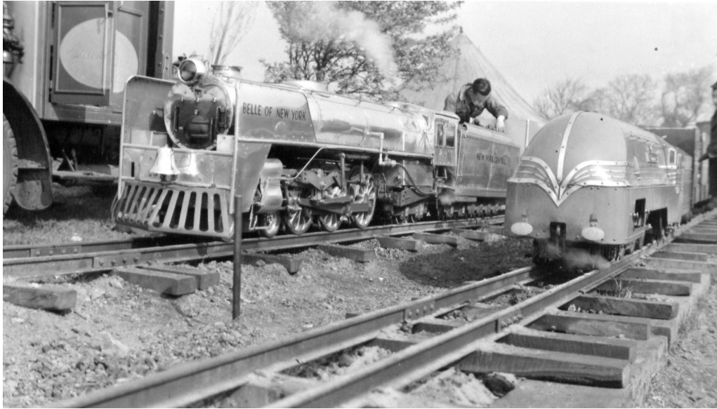
The first stop on the 1948 tour was at Exhibition Park in Newcastle. Here we see Ken Dove preparing "Belle of New York", with "Coronation" alongside. Note the lorry on the left and the model exhibition marquee behind Ken Dove. For its first year "Belle of New York" was finished in unpainted polished aluminium, as seen here. Note the method of track laying. ( Courtesy Charlton Collection, Beamish Museum )
