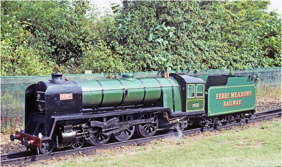
"Henry" "Commodore Vanderbilt" was rebuilt into this attractive, LNER style, 4-6-2 by Alec Mills. It was later named "Henry" and regained its original number of 1950. It ran for many years on the Ferry Meadows Railway at Peterborough, where it is seen here.
