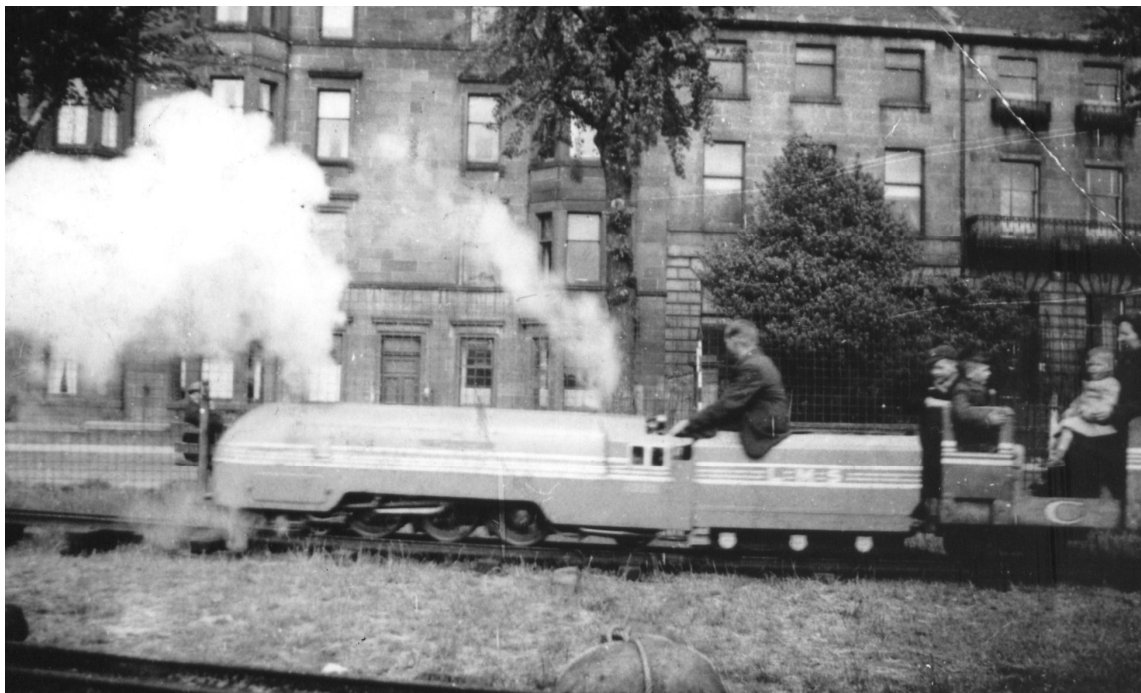
"Coronation" has reached the end of the track at Leith Links, Edinburgh in May 1948. Note how the end of the track is ramped up and the large sand bag on the nearer track. The terraced houses in the background are in James Place (now Links Gardens) - the door directly above the leading driving wheel of "Coronation" is the present day No.5A. This view also clearly shows how the coaches were painted to match "Coronation". ( Courtesy S. Townsend Collection )
